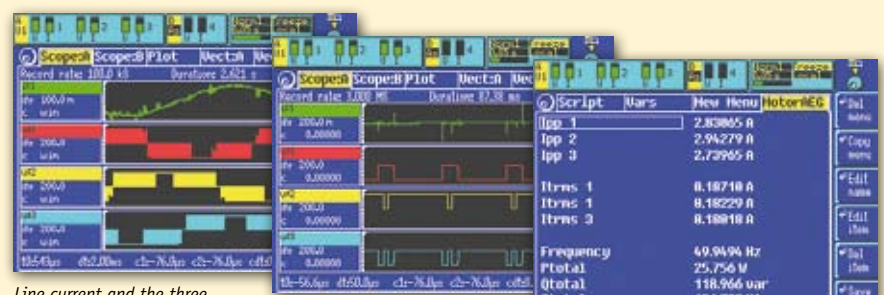
Extra high current peaks at simultaneous switching edges
