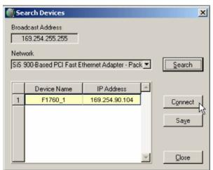
Your instrument will show up in the list. Press **Connect** to establish a connection between Fluke 1760 and your computer. The status line shows information about the connection.
